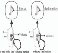
press and hold the Volume button for 5 seconds
